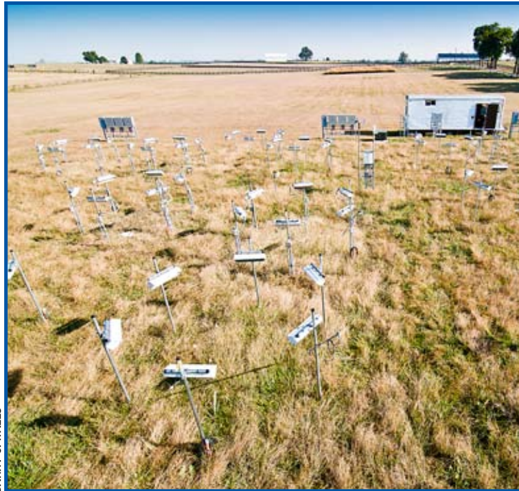
Researchers use infrared radiant heaters to warm the air.
